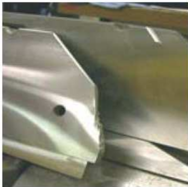
Abused fence - blade impact
