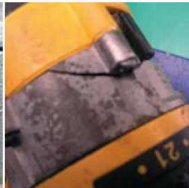
Cracks on dropped unit
